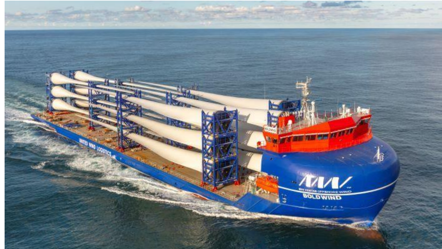
Wind Turbine component transport vessel “Bold Wind” transporting blades for 5 offshore turbines
